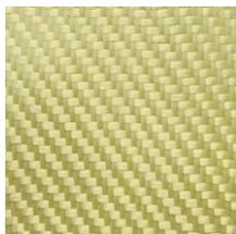
When combined with other reinforcements (glass, carbon), it offers excellent resistance to puncture. The infusion process plays a crucial role in preventing water absorption. Like carbon, adding **Kevlar** reduces the quantities of resin involved.
