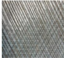
To overcome the deficiencies of linen while achieving more virtuous production, a glass / linen hybrid is under development. It is scheduled to be tested in early 2021. In all likelihood, it will be used for the interior counter moldings. Note that linen has a carbon footprint **6 times lower** than that of glass if only the product is considered. In terms of grey energy\*, the gain is only 15%.
